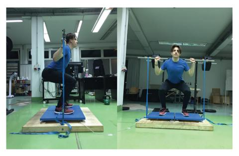
**Figure 1.** The set-up and positioning during isometric MVC tasks. The length of the bands was adjusted to ensure 30°, 60° and 90° knee angles.
