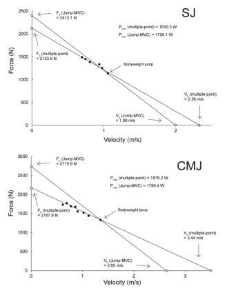
**Figure 2.** Graphical representation of F–V profiling for a sample subject using multiple-point method and Jump-MVC method, using mean force data from the 30, 60 and 90° angles. SJ–Squat jump, CMJ– countermovement jump,  $F_0$ –maximal force,  $V_0$ –theoretical maximal velocity,  $P_{max}$ –maximal power.
