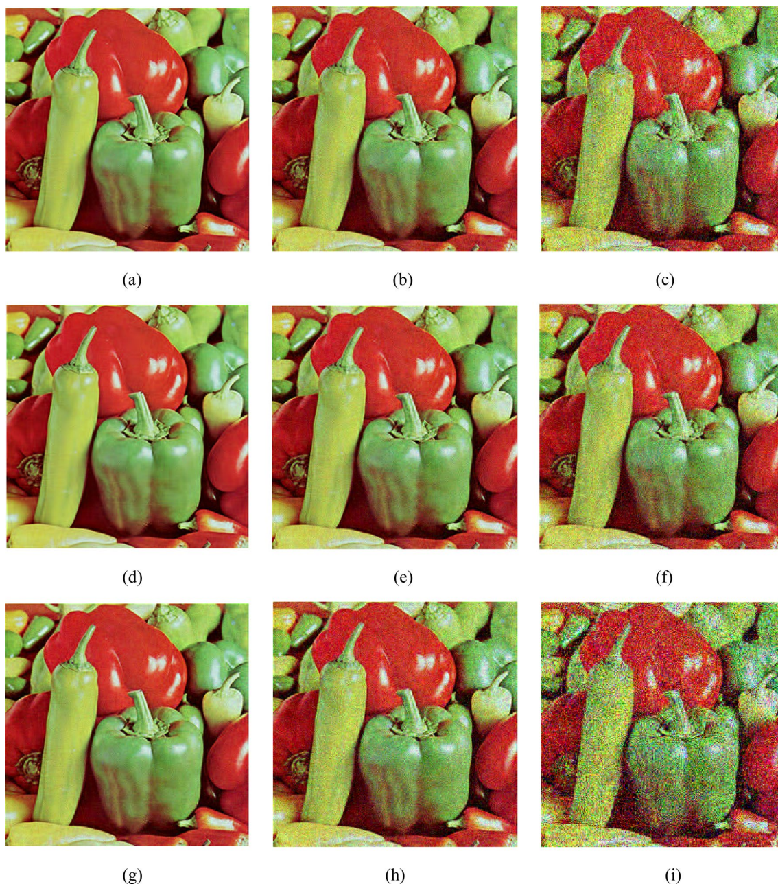
Figure 8. The results of noise attack with different noise strengths: (a) 10^{-5} GN, (b) 10^{-4} GN, (c) 10^{-3} GN, (d) 10^{-4} SPN, (e) 10^{-3} SPN, (f) 10^{-2} SPN, and (g) 10^{-4} SN, (h) 10^{-3} SN, (i) 10^{-2} SN.
