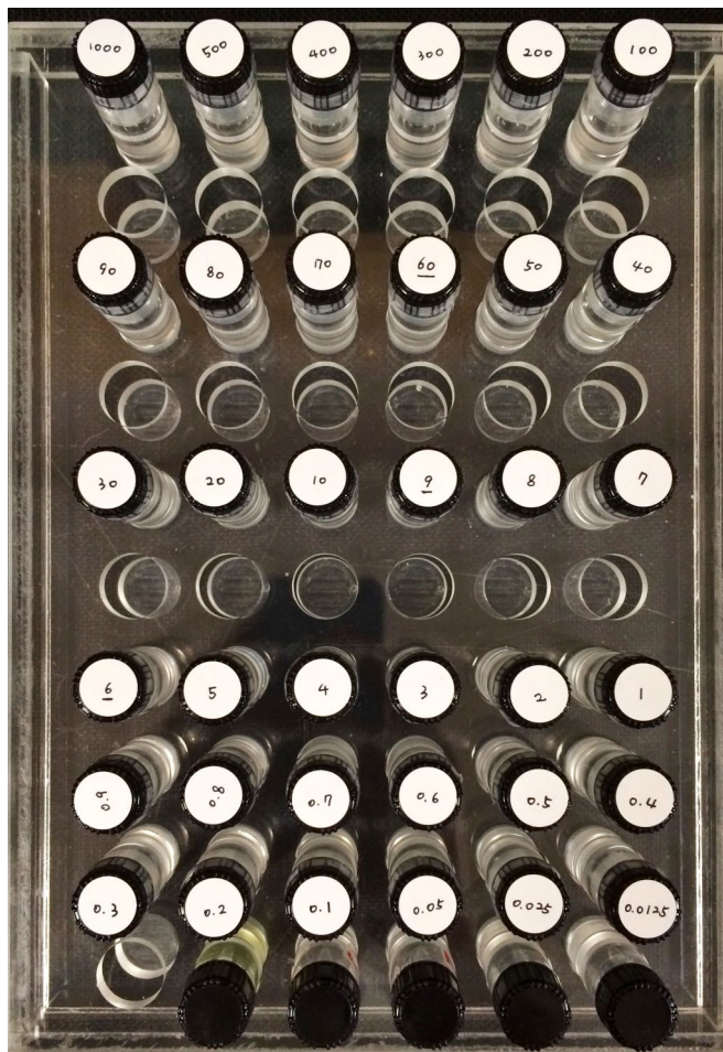
Figure 5. Phantom objects. Phantom tubes containing multiple vials of various Gadoterate meglumine concentrations.
