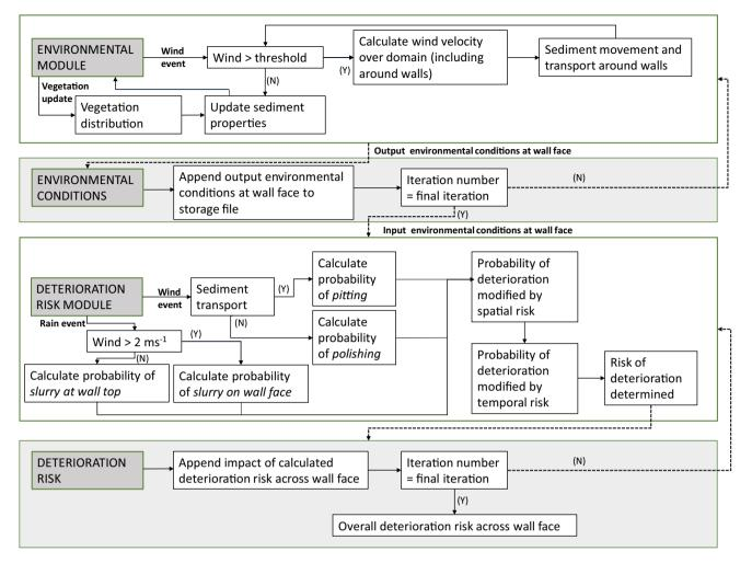
**Figure 4.** A schematic of the environmental and deterioration risk modules within ViSTA-HD. Reproduced with permission<sup>21</sup>.
