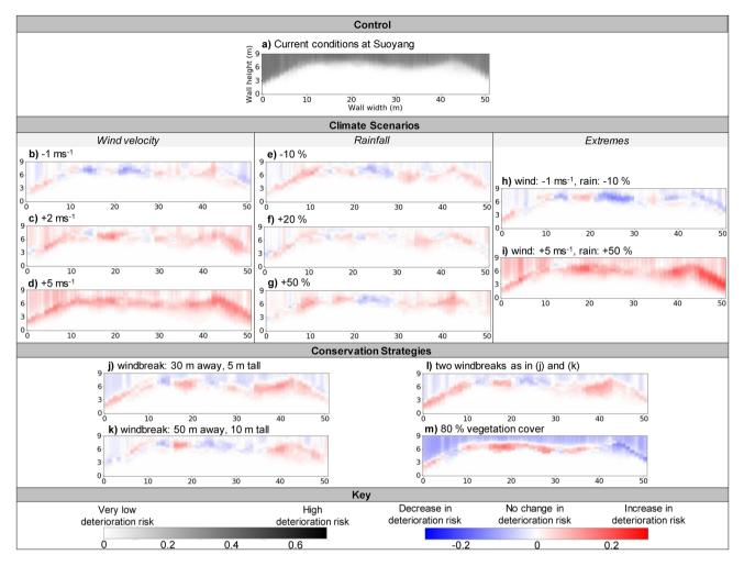
**Figure 2.** The overall risk of deterioration after 100 years under: (a) current climatic conditions; (b–i) different climatic changes; and (j-m) different conservation strategies. In panels (b-m), deviations from the control results are shown with red and blue, indicating an increased and decreased risk of deterioration, respectively.
