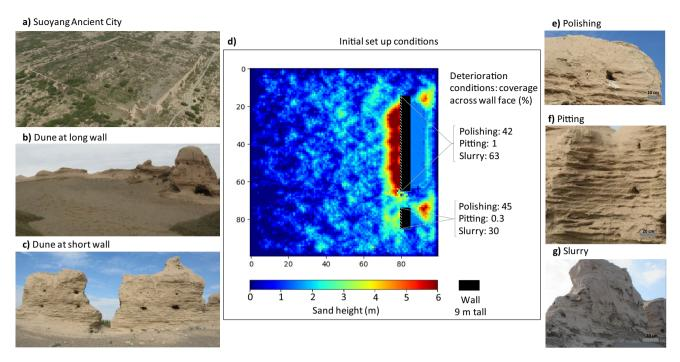
**Figure 1.** The site of Suoyang Ancient city (a-c), a plan view of the initial model setup (d) and the three major deterioration features (e-g).
