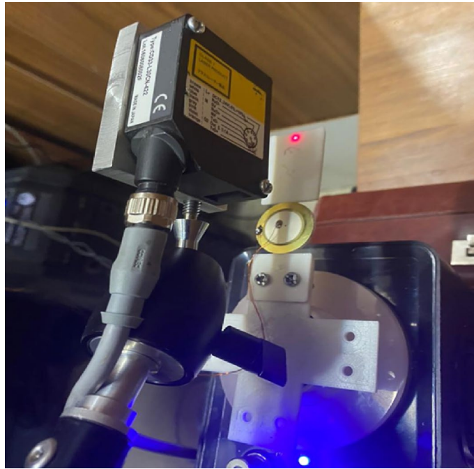
Figure 10. Top view of the experimental setup for the vibration energy harvesting system.
