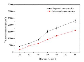
**Figure 12.** Comparison between calculated and measured concentrations in the chamber. The error bars shown with the expected concentration values were calculated by propagating the individual uncertainties associated with soil gas flow rate ( $\pm 4\%$ ) and soil gas <sup>222</sup>Rn concentration ( $\pm 3\%$ ).
