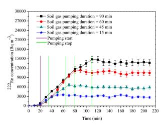
**Figure 10.** The build-up of  $^{222}$ Rn concentration achieved in the chamber for a fixed flow rate of 60 L min<sup>-1</sup>. Duration of injection varied from 15 to 90 min.
