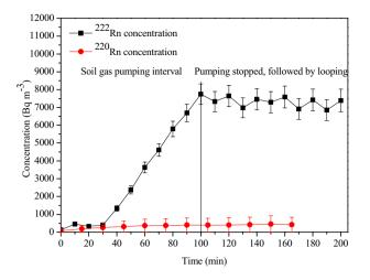
**Figure 6.** Concentration profiles of <sup>222</sup>Rn and <sup>220</sup>Rn in the chamber after pumping soil gas (<sup>222</sup>Rn measurements by AlphaGuard and <sup>220</sup>Rn by Smart RnDuo).
