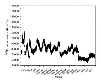
**Figure 4.** Variation of <sup>222</sup>Rn concentrations in soil gas for 1 year (measured using scintillation cell-based online <sup>222</sup>Rn monitor).
