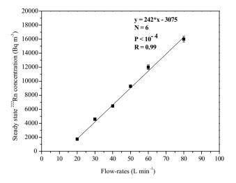
**Figure 11.** Correlation between the steady-state <sup>222</sup>Rn concentrations attained in the chamber with the soil gas pumping rates (for a fixed pumping duration of 60 min).
