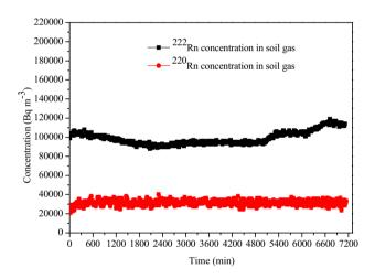
Figure 5.  $^{222}$ Rn and  $^{220}$ Rn concentrations profiles in soil gas measured at the outlet of the soil probe.
