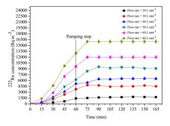
**Figure 9.** The build-up of <sup>222</sup>Rn concentration inside the chamber at various injection rates for a fixed injection time of 60 min.
