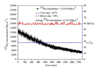
**Figure 8.** Illustration of the application of soil gas for the static mode operation of the chamber. One-time filling of the chamber with <sup>222</sup>Rn and the experiments are performed during the decay of <sup>222</sup>Rn.
