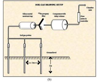
**Figure 2.** Schematic diagram of (**a**) calibration chamber and soil gas harvesting set-up (**b**) expanded view of soil gas harvesting set-up.
