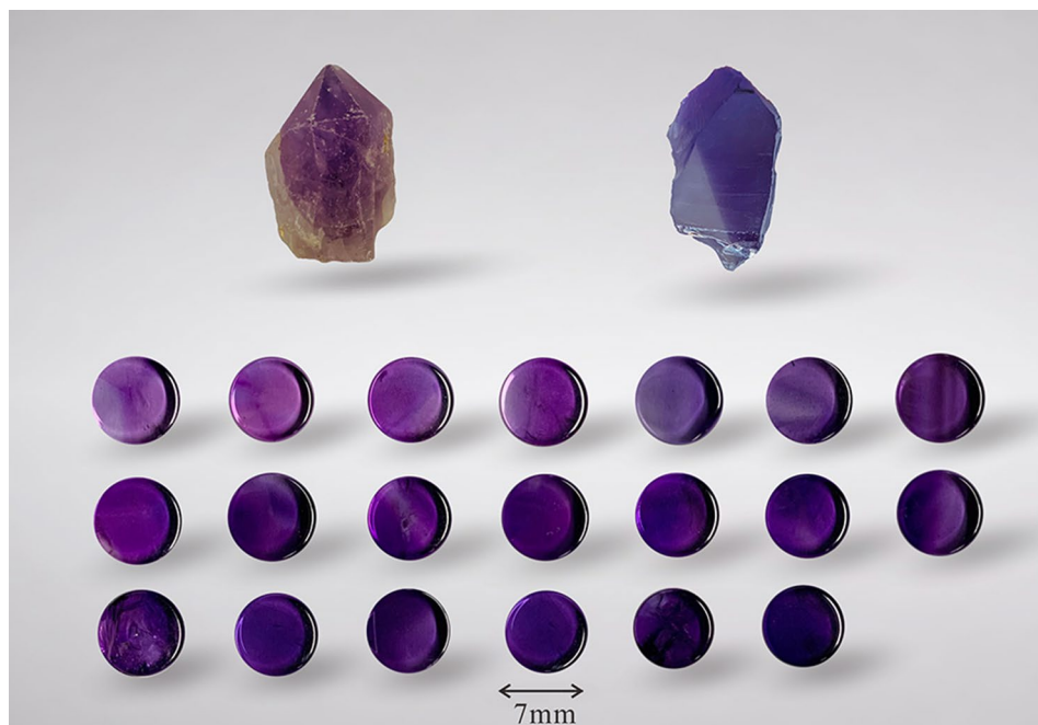
Figure 1. The picture of samples. Round flat samples which are used for color parameters testing have an average weight of 4.01 g and the raw stones at the top of the picture are used for XRD measurement. The lightness of these samples ranges from 21.99 to 53.47, the chroma ranges from 31.80 to 51.25 and the hue angle ranges from 312.1 to 322.5. The figure was taken and drawn by Renping Cheng using CorelDRAW Graphics Suite X8 2016 18.0.0.405 ( https://www.corel.com ).
