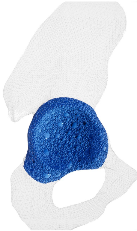
Figure 8. Example of a volumetric model of the acetabulum filled with spheres, which is used to calculate the force feedback given by the Virtual Reality simulator. The usage of spheres allows a fast computation of the force feedback.
