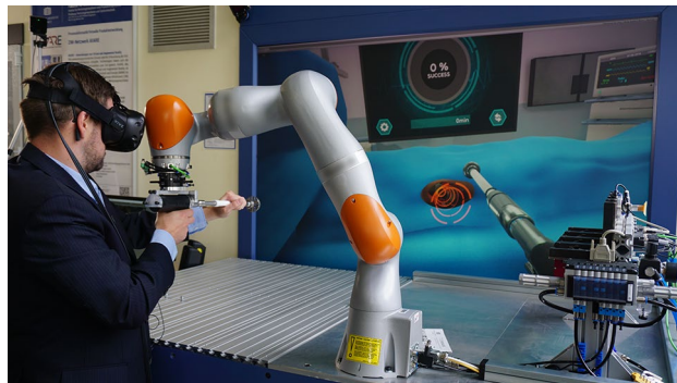
Figure 9. The Virtual Reality acetabulum reaming simulator, where the developed real-time material model is used to simulate the interactional forces and torques between the reamer and the acetabulum.
