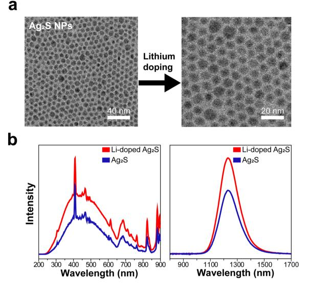
**Figure 2.** Synthesis of  $Ag_2S$  NPs and Li-doped  $Ag_2S$  NPs. (a) Representative TEM images of  $Ag_2S$  NPs (left) and Li-doped  $Ag_2S$  NPs (right) with a 10 nm size. (b) PL excitation spectra (left) and emission spectra (right) under excitation from an 850 nm light source.
