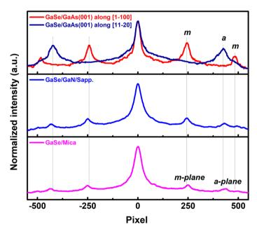
Figure 3. RHEED intensity profiles of the GaSe layers on various substrates.
