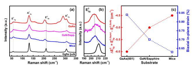
**Figure 5.** (a) Raman scattering spectra of GaSe bulk and GaSe films grown on various substrates, (b) An enlarged Raman spectra near  $E_{2g}^2$  peaks, and (c) Biaxial in-plane lattice strain of these GaSe layers extracted from the red-shift of  $E_{2g}^2$  Raman active mode.
