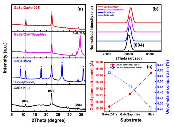
**Figure 4.** Long-range (**a**) and near (004) peak (**b**) XRD 2θ-scans of GaSe bulk and GaSe films grown on various substrates. (**c**) Out-of plane lattice constants and compressive strains of GaSe layers.
