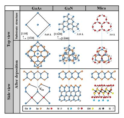
Figure 2. Illustration of perspective atomic-stacking configuration between GaSe layers and substrates.
