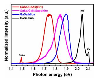
Figure 6. PL spectra of the GaSe epilayers on various substrates in comparison to GaSe bulk measured at 10 K.
