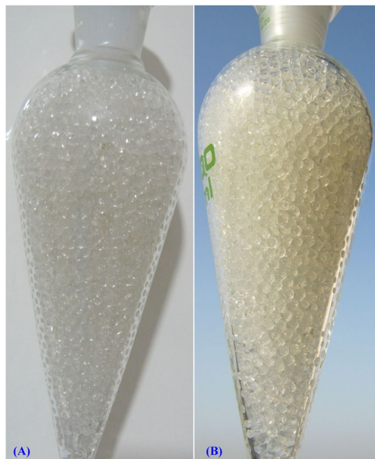
Figure 9. Immobilization of Azotobacter nigricans NEWG-1 in alginate beads during \text{Cu}^{2+} ions removal from aqueous solution. (A) Separating funnel packed with alginate beads, (B) Separating funnel packed with alginate- Azotobacter nigricans NEWG-1 beads.
