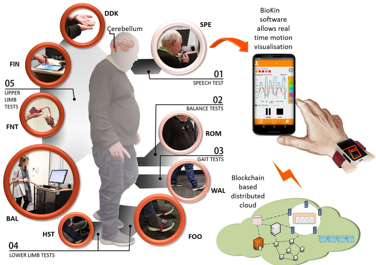
Figure 1. BioKin cloud based real time motion capture sensor platform designed for objective assessment of ataxic movements ranging from speech to lower body kinematics. Repeated syllable utterance (SPE), stance/romberg (ROM), gait (WAL), foot tapping (FOO), heel-shin (HST), ballistic tracking/finger-chase (BAL), finger-nose/nose-finger (FNT), rhythmic finger tapping (FIN), dysdiadochokinesia (DDK) are the instrumented tests.
