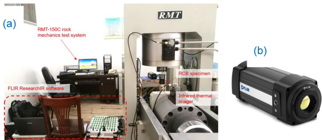
Figure 6. UCT equipment (a) RMT-150C electro-hydraulic servo rock mechanics test system (b) FLIR infrared thermal image monitoring system.
