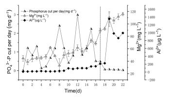
**Figure 4.** The PO<sub>4</sub><sup>3-</sup>-P reduction amount per day and Mg<sup>2+</sup>, Al<sup>3+</sup> ions concentrations in the purification of eutrophic water by EEFBs, data points represent sample means  $\pm$  the standard error of the mean.
