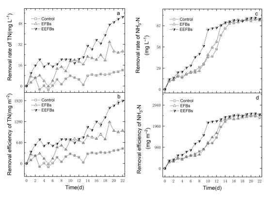
**Figure 2.** The removal rates and removal efficiencies of TN (**a**,**b**) and NH<sub>3</sub>-N (**c**,**d**) in the EEFBs and the EFBs during the purification of eutrophic water, data points represent sample means  $\pm$  the standard error of the mean.
