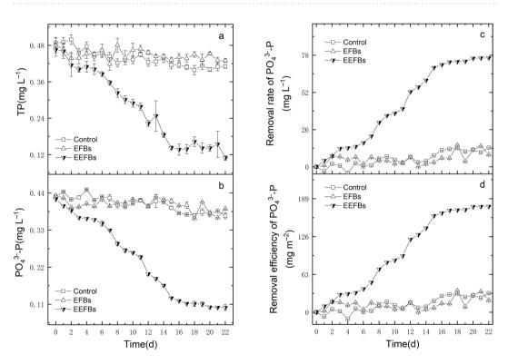
**Figure 3.** The concentrations of the TP (**a**) and  $PO_4^{3-}$ -P (**b**), removal rates of  $PO_4^{3-}$ -P (**c**) and removal efficiency of  $PO_4^{3-}$ -P (**d**) during the purification of eutrophic water, data points represent sample means ± the standard error of the mean.
