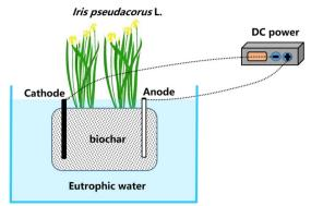
Figure 8. Schematic diagram of electrolysis-ecological floating bed (EEFB).
