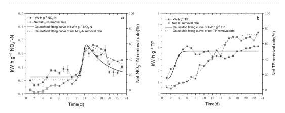
**Figure 7.** The electrolysis power consumption and net removal rates of TN (**a**) and TP (**b**) by the EEFBs during the purification of eutrophic water.
