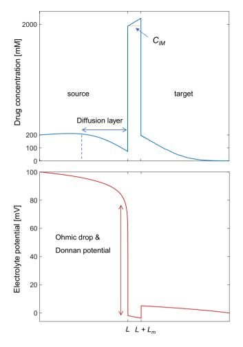
**Figure 2.** Snapshots of drug concentration (top) and voltage (bottom) profiles at t = 20 s. Initial drug concentration  $C_D$  is 200 mM, and fixed charge concentration  $C_{IM}$  is 2 M. Reservoir length  $L = 100 \,\mu\text{m}$  and membrane thickness  $L_m = 10 \,\mu\text{m}$ .
