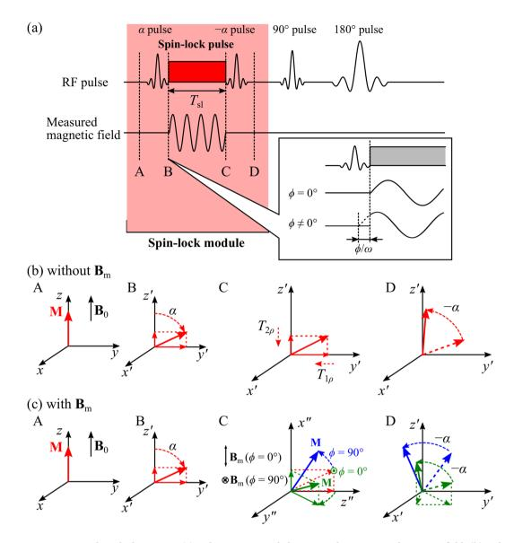
**Figure 1.** Partial spinlock sequence (a) and magnetisation behaviour without measured magnetic fields (b) and with measured magnetic fields of the phase difference between the measured magnetic field and the spinlock pulse  $\phi = 0^{\circ}$  and 90° as examples (c).
