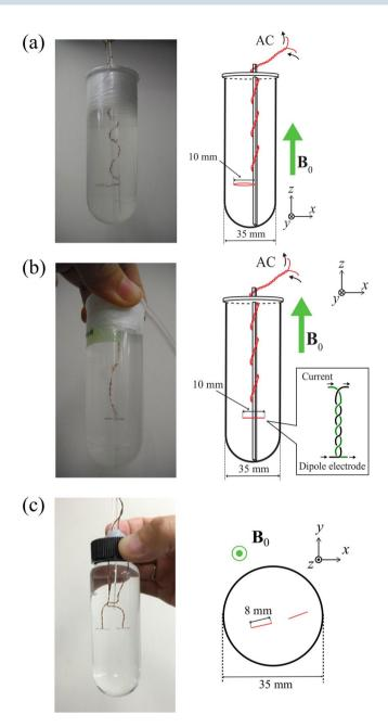
**Figure 2.** Phantoms used in experiments. (a) Photograph (left) and illustration (right) of the loop-coil phantom (b) Photograph (left) and illustration (right) of current-dipole phantom (c) Photograph (left) and illustration (right) of current-dipole phantom containing two dipole electrodes. The coil and the dipole electrodes were held with an acrylic rod in a normal saline solution.
