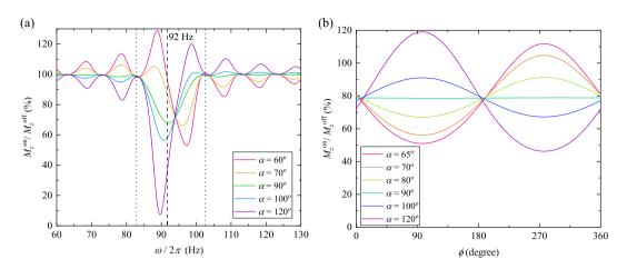
**Figure 3.** Simulated MR signal changes as a function of (a) the frequency of the measured magnetic fields and (b) the initial phase  $\phi$  with various  $\alpha$ . (a) The flip angle  $\alpha$  was varied from 60 to 120 degrees. The magnetic field  $B_{\rm m}=50$  nT, the spinlock frequency  $\omega_{\rm sl}/2\pi=92$  Hz, and  $\phi=0^{\circ}$ . (b) The magnetic field  $B_{\rm m}=40$  nT, and the frequency  $\omega/2\pi$  and the spinlock frequency  $\omega_{\rm sl}/2\pi$  were 88 Hz.
