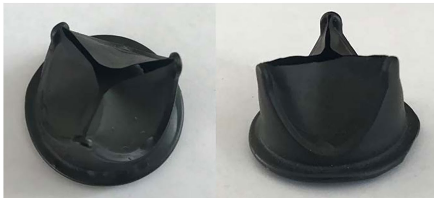
Figure 10. A prototype of polymeric heart valve made from Hastalex.
