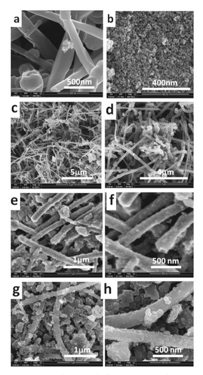
**Figure 3.** NanoSEM photomicrographs of MWCNTs/RFA-CNp with 50/50 g/g mixing ratio at different mixing times and different scales of magnifications. (**a,b**) refers to pristine MWCTs and CNp, respectively. Each couple of photomicrographs of (**c,d**) 0D, (**e,f**) 185D and (**g,h**) 415D refer to different scales of magnifications for the corresponding sample.
