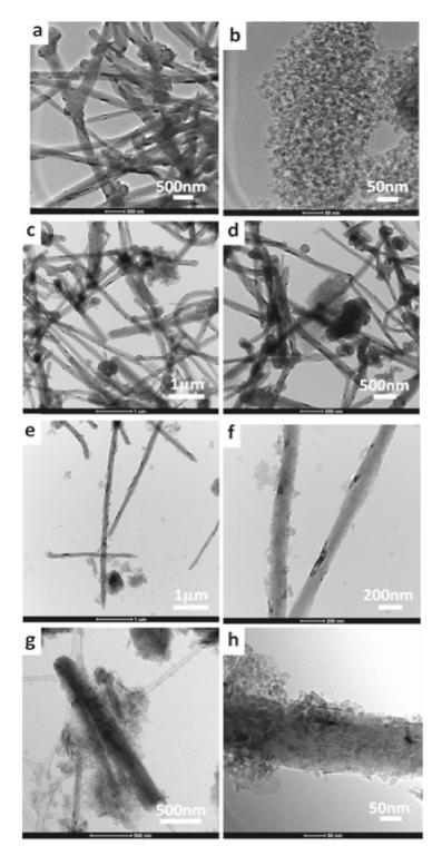
**Figure 4.** TEM photomicrographs of MWCNTs/RFA-CNp with 50/50 g/g at different aqueous mixing time of stirring and different scale of magnification. (**a,b**) refers to pristine MWCTs and CNp, respectively. Each couple of photomicrographs of (**c,d**) 0D, (**e,f**) 185D and (**g,h**) 415D refer to different scale of magnifications.
