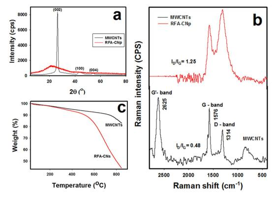
**Figure 1.** (a) XRD patterns, (b) Raman spectra and (c) TGA thermograms of MWCNTs (black line) RFA-CNp (red line) samples.
