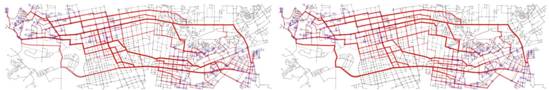
Figure 7. Results in Sendai city obtained by (Upper panel) the shortest-path policy and (lower panel) our method. The color strength of the red color on each road denoted by the edges represents the number of cars passing it. The blue points are the starting and destination points. We test our method around the point with 38^{\circ}28' north latitude and 140^{\circ}92' west longitude.
