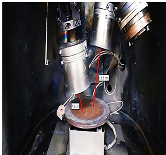
Figure 2. Physical view of the pinhole reduction technique.
