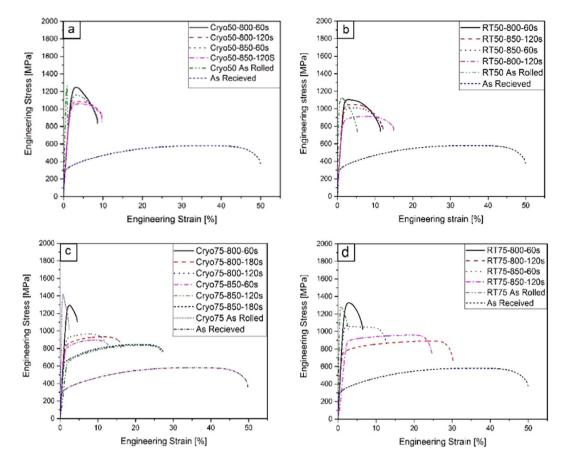
**Figure 2.** Stress-strains curves of rolled UNS S31000 stainless steel by Cryo- and room temperature rolling to 50% and 75% thickness reduction. (Refer to online version for colour reference).
