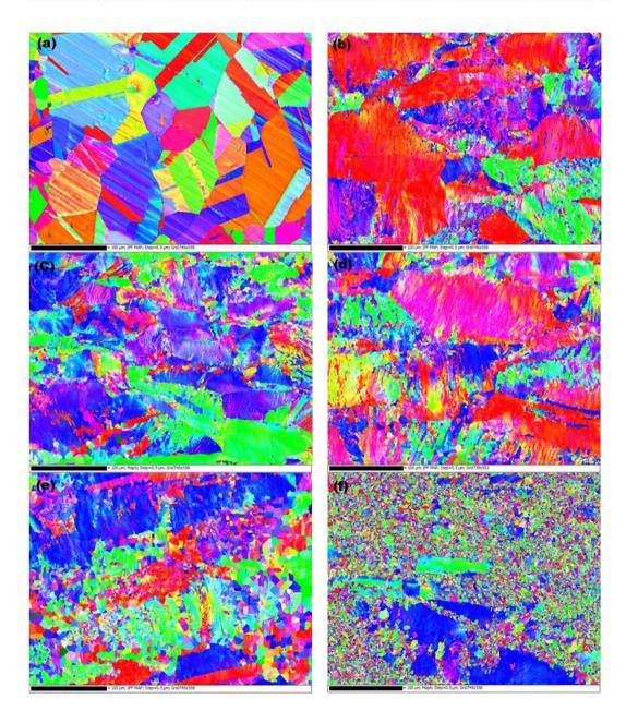
**Figure 4.** Inverse pole figure maps; (**a**) as received, (**b**) RT50, (**c**) Cryo50, (**d**) Cryo50 Annealed (**e**) Cryo75 and (**f**) Cryo75 Annealed conditions comparing grain size and crystallographic orientation.
