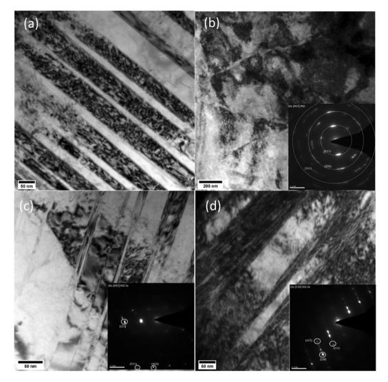
**Figure 6.** TEM micrographs of (**a**,**b**) Cryorolled 50%, (**c**) 75% thickness reduction and (**d**) Room temperature rolled sample of 50% thickness reduction.
