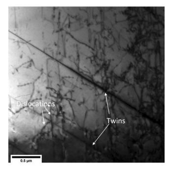
**Figure 5.** TEM micrograph of as-received sample showing relatively low dislocation density and widely spaced twins.
