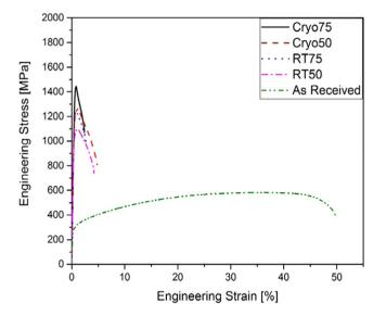
Figure 1. Effect of Cryo- and room temperature rolling on the stress-strain behaviour of UNS S31000 stainless steel.
