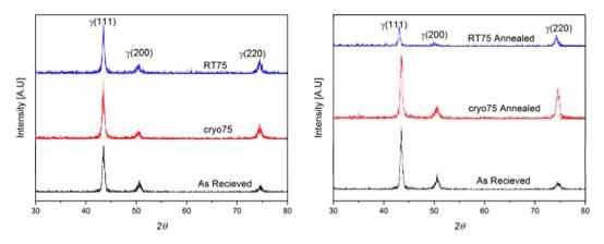
Figure 3. X-Ray diffraction patterns; (a) Rolled samples and (b) Rolled and annealed samples.
