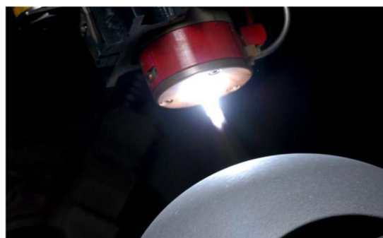
Figure 4. Plasma Coating Process-The figure describe the Piston and head coated by CUCr1Zr material (Own Image -Photograph taken by corresponding author at the time of piston coating at Bangalore).
