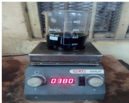
Figure 7. Blending of Cotton Seed bio oil mixing with Diesel Fuel – The figure shown cotton seed bio oil stirring with diesel fuel and heating. (Own Image -Photograph taken by corresponding author at the time of research work).
