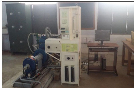
Figure 6. Experimental setup –The Engine Connected with Eddy Current Dynamometer and Exhaust Gas Analyzer (Own Image -Photograph taken by corresponding author during experiment conducted).
