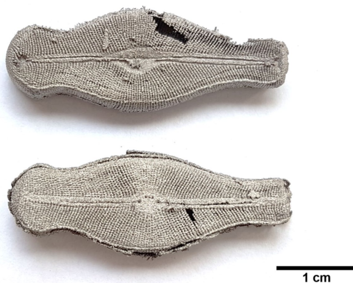
Figure 5. 3D printed engineered object made of titanium, based on the natural diatom frustule design.
