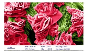
**Figure 7.** FE-SEM image for top phase with the nanoparticle. The red color represents vanillin + PEG and the green color represents functionalized MWCNT.
