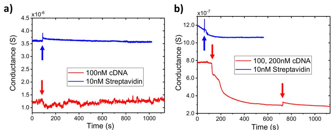
**Figure 5.** Biosensor response to different analytes. Conductance vs. time plots of bare (a) and Au NP decorated (b) single ZnO NW devices upon introduction (arrows) of 10  $\mu$ L of the indicated solution. Au NP decorated biosensors respond to multiple analytes after functionalization with the same DNA aptamer. Increased analyte concentration results in a proportionally larger change in Au NP decorated NW conductivity, until saturation of all available Au NP sites.
