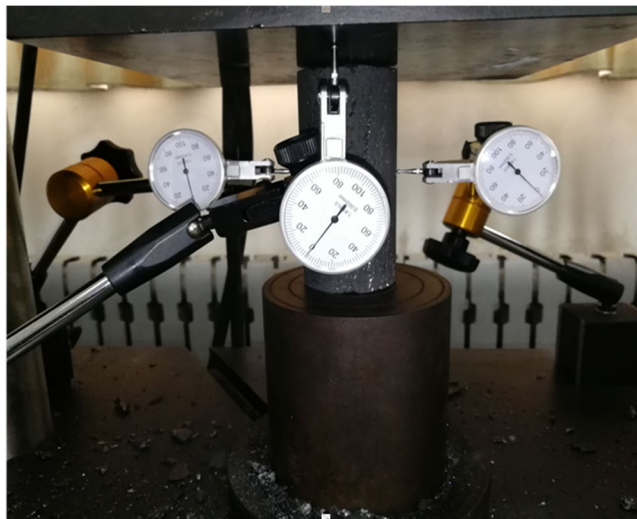
Figure 4. Schematics of compressive strength test.
