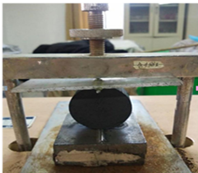
Figure 5. Schematics of tensile strength test.
