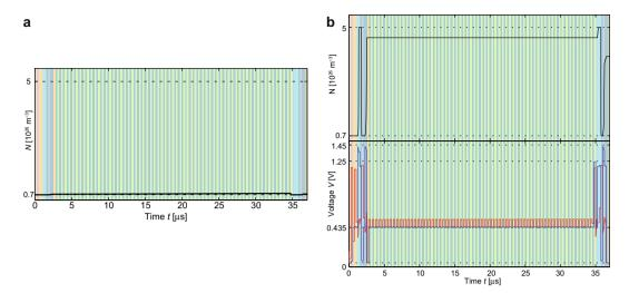
**Figure 6.** Simulation and comparison of the multibit adder. (a) State variable of  $S_{WL65}$  under the worst case conditions. The worst case is found to be A – B, where A is 0 and B is 0. The color scheme is adopted from Fig. 3. (b) State variable and applied voltage of  $M1_{WL65}$  for the worst case simulation. The potential of the wordline is depicted in red and the potential of the connection point at the bitline is shown in blue.
