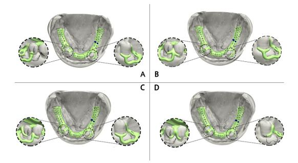
Figure 4. 4 Different designs of frameworks.
