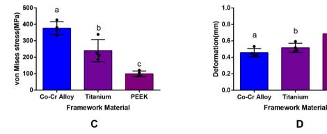
Figure 1. Max von Mises stress values and displacement of models under vertical loading.
