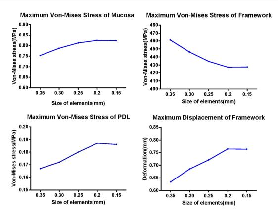
Figure 6. Convergence study: Influence of the size of elements on maximum Von-Mises stress and maximum displacement of finite element model.
