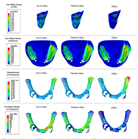
Figure 2. von Mises stress of PDL, mucosa, framework and displacement of framework under vertical loading.
