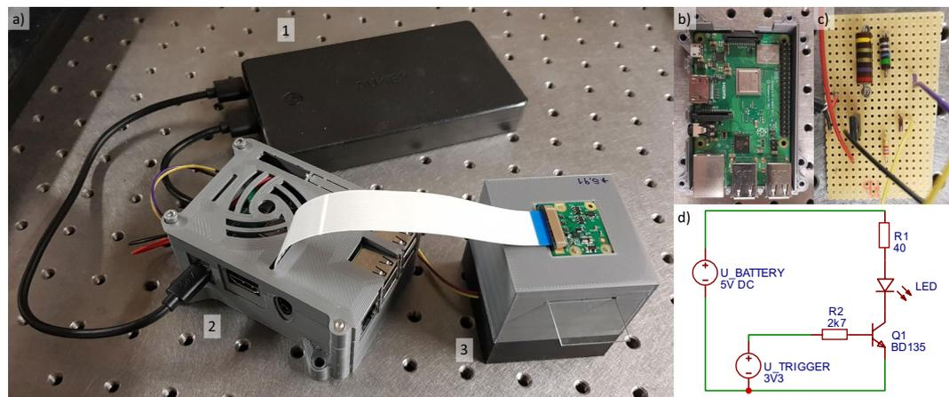
**Figure 5.** (a) The fully portable DIHM system consisting of (1) USB-port power bank, (2) 3D printed housing containing Raspberry Pi and LED control circuit, (3) LED DIHM system as presented in Fig. 1(d). (b) Closeup of the Raspberry Pi single-board computer. (c) Closeup of the LED control circuit. (d) Schematic of the circuit for biasing the LED using the Raspberry Pi's GPIOs.
