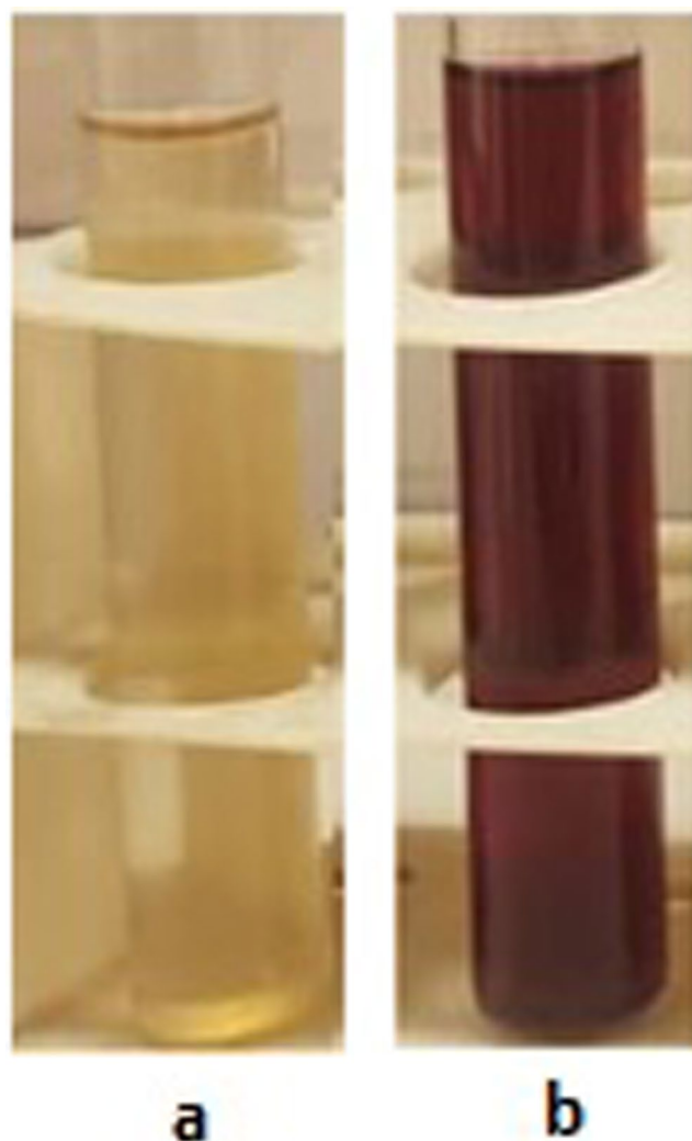
Figure 1. The obtained color changed supernatant due to the GNPs production. (a) Fungal culture supernatant before GNPs production and (b) Fungal culture supernatant after GNPs production.
