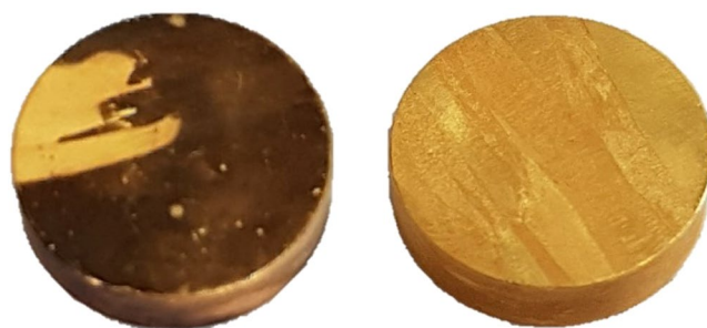
Figure 12. Gold specimen in cyanide test (0.14 M KCN) after 3 h (left) and after 6 h (right picture).
