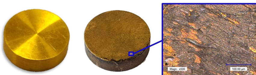
Figure 5. Passivation of gold surface in thiosulfate leaching experiments (from left to right: initial sample, 65 °C after 8 h leaching, optical microscopy magnification x500).
