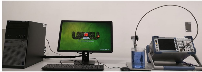
Figure 1. Microwave dielectric measurement setup consisting of an open ended coaxial probe, a vector network analyzer (VNA) and an external computer. Microwave signals generated by the VNA were transmitted via the coaxial cable to the probe tip submerged in the sample under test. Signals backscattered from the samples were analyzed using the DAK software installed in the computer to extract the dielectric parameters.
