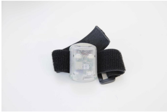
Figure 1. ABBI, the Audio Bracelet for Blind Interaction, is a small wearable custom-designed technology with integrated audio system, motion sensors, and a Bluetooth low energy module to communicate with a smartphone. The core idea behind ABBI is to use the auditory modality to convey spatial information about the movement of the person's own body within the personal, peri-personal and extra-personal space.
