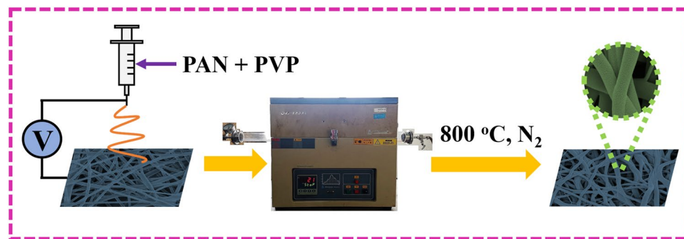
Figure 1. Synthesis schematic diagram of carbon nanofibers with adjustable nanostructure.
