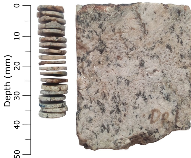
Figure 5. Photograph of a sliced rock core used for conventional RSD measurements (left). Photograph of the rock slab used for the HR-IRPL measurements (right).
