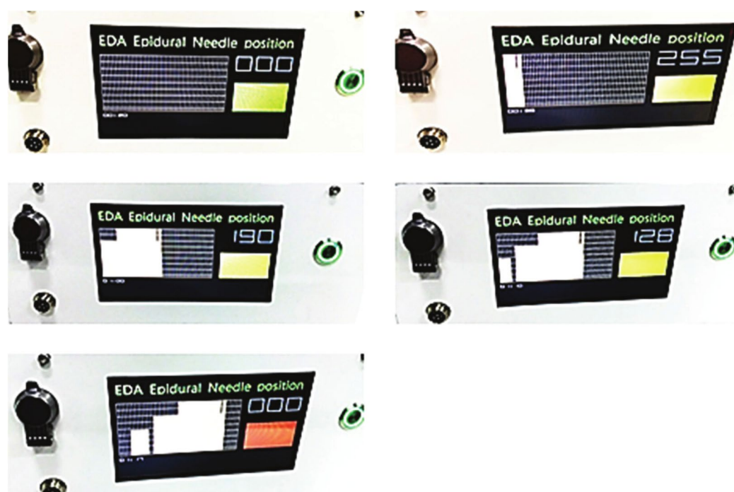
Figure 3. Optical-guided Location Device data displays. When reflection intensity is 0 meaning no reflected light received, in this case color bar will be green; When reflection intensity reaches 255 the color bar will turn yellow meaning needle tip has reached fat layer tissue; When reflection intensity decreases with advance of needle tip and drops to zero color bar will turn red bar indicating that the needle tip has reached the epidural space.
