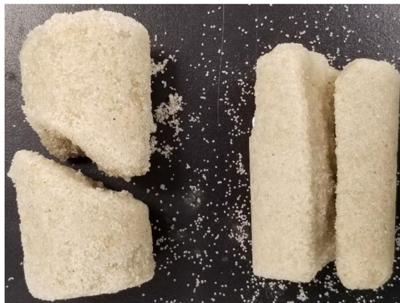
Figure 2. Failure patterns of EICP-treated specimens: shear failure of specimens treated with baseline solution (no powdered milk) (left); and tensile splitting of specimens treated with modified solution (with powdered milk) (right).
