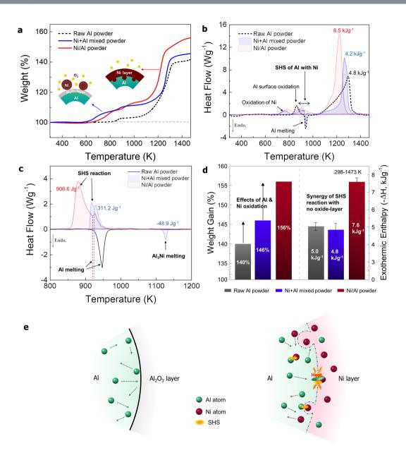
**Figure 3.** (a) TGA and (b) DSC results with increasing temperature in air atmosphere (heating rate of  $10 \,\mathrm{K\,min^{-1}}$ ), (c) changes in heat flow as a function of temperature in Ar atmosphere (heating rate of  $10 \,\mathrm{K\,min^{-1}}$ ), (d) comparison of weight gain and exothermic enthalpy energy of fine Al particles, mixed powder, and Ni/Al powder, (e) schematic illustration of SHS reaction in activated Ni/Al interface compared to that in surface-passivated Al.
