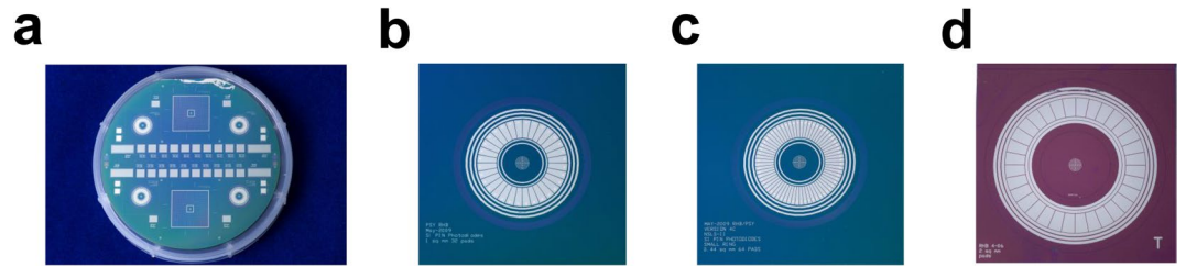
Figure 4. Prototype sensors. (a) A finished Si wafer containing four 32-segment diode rings arranged in each quadrant. (b) [Prototype-II-32] A fully optimised layout of the photodiode ring array composed of 32 segments, each having its surface area of 1.0 \text{ mm}^2 . (c) [Prototype-II-64] A ring array of the 64 diode segments, each measuring 0.44 \text{ mm}^2 . (d) [Prototype-I-32] An unoptimised version of the 32-segment diode array.
