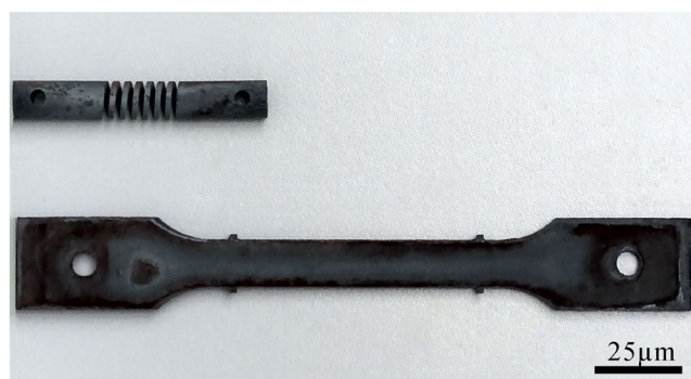
Figure 11. Helical spring and rectangular specimens following thermal treatment.
