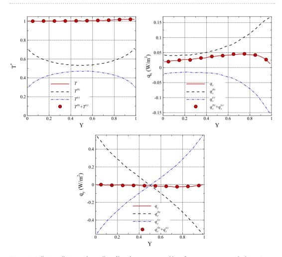
**Figure 2.** Ballistic, collision, and overall profiles of temperature and heat flux components over the line x/L = 0.5 in case Kn = 1.
