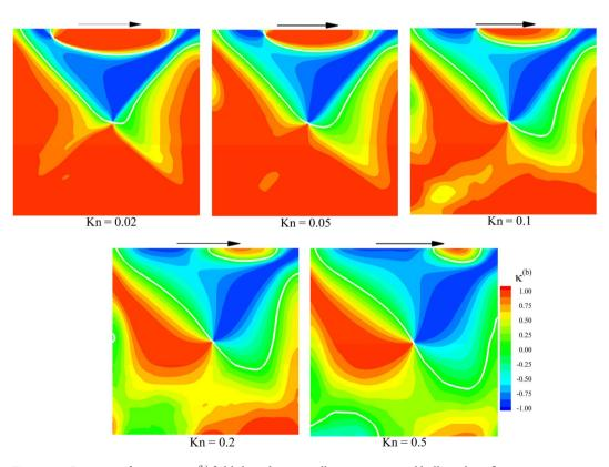
**Figure 6.** Contours of parameter  $\kappa^{(b)}$  fields based on overall temperature and ballistic heat flow.
