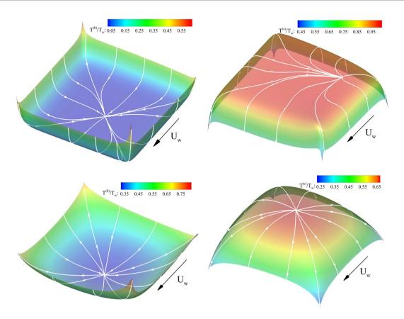
**Figure 4.** Ballistic heat flow lines overlaid on the ballistic temperature field (left) and collision heat flow lines overlaid on the collision temperature field (right) for Kn = 0.05 (up) and Kn = 0.5 (down).
