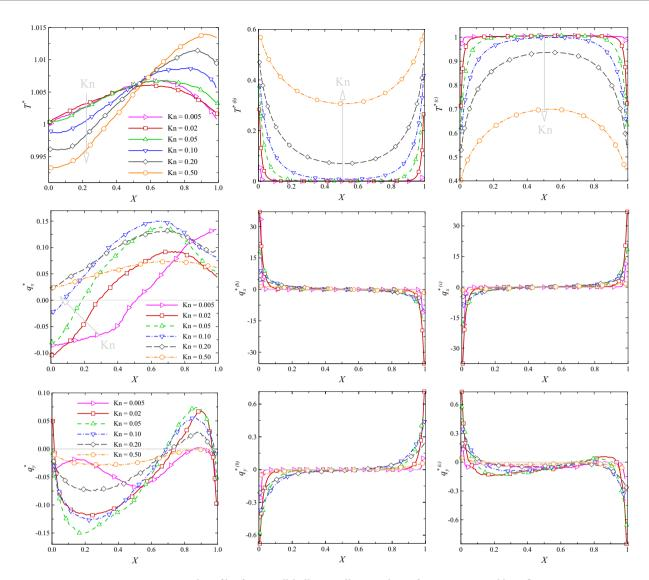
**Figure 9.** Horizontal profiles for overall/ballistic/collision values of temperature and heat flux components at y/L = 0.5 at various Knudsen numbers.
