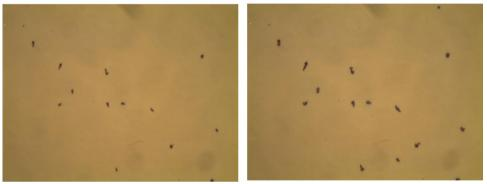
**Figure 5.** Optical microscope images (100X magnification) recorded at the same spot over time showing ripening of 3 nm BCP clusters on an ITO surface.
