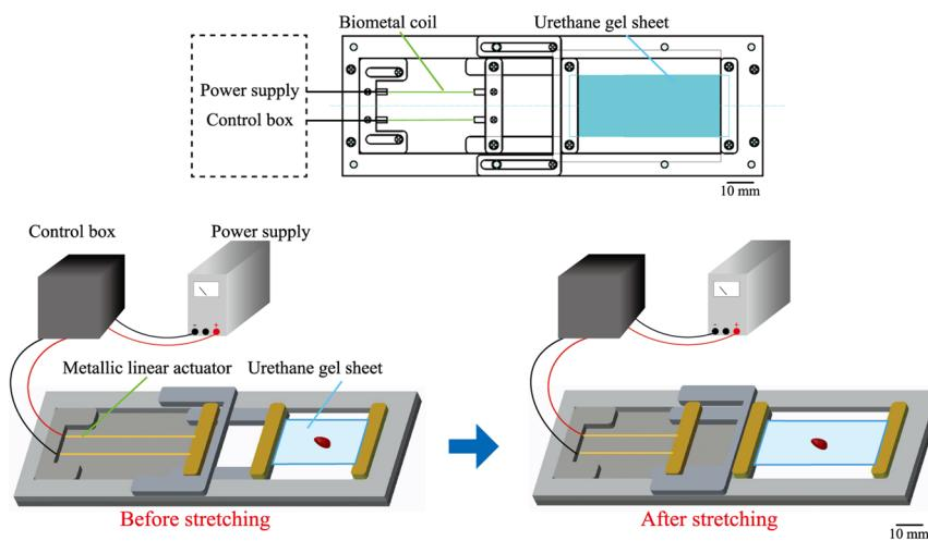
**Figure 1.** Schematic representation of the experimental set-up used to stretch a tissue slice attached to a gel sheet on the stage of an optical microscope.
