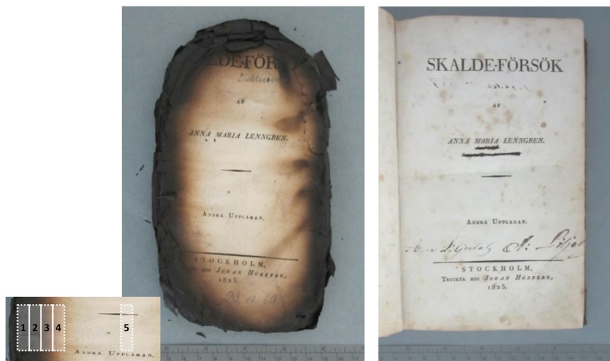
Figure 8. Book papers analyzed in the study. Left - burned book by the fire at the Duchess Anna Amalia Library in 2004. The lower left image indicates where the samples were taken (5-center; 4- light brown; 3-brown; 2-dark brown; 1-black brown). Right – not-burned identical book.
