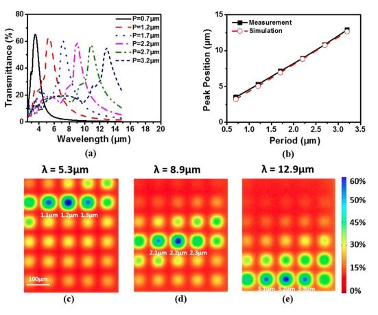
**Figure 3.** (a) Experimentally measured optical transmission spectra of six (out of 30 in total) microhole arrays. (b) Transmittance peak position as a function of the aperture period in simulation and experimental results. Mid-infrared transmission 2D maps of the MHAs are plotted at three different wavelengths:  $5.3 \,\mu m$  (c),  $8.9 \,\mu m$  (d) and  $12.9 \,\mu m$  (e).
