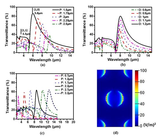
**Figure 1.** (a) Simulations as periodicity changes from  $1.5 \,\mu\text{m}$  to  $2.5 \,\mu\text{m}$  at a fixed diameter of  $1 \,\mu\text{m}$ . (b) Simulations as diameter changes from  $0.8 \,\mu\text{m}$  to  $1.2 \,\mu\text{m}$  at a fixed periodicity of  $2 \,\mu\text{m}$ . (c) Simulation results of Au MHAs with a fixed ratio 0.5 for aperture diameter to period. (d) Top view of the simulated E-field distribution inside the holes at peak position.
