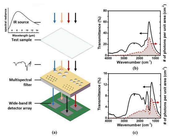
**Figure 4.** (a) IR spectrometric analyzer model using microhole array multispectral filters. Transmission spectrum of a microhole array ( $P = 1.7 \mu m$ ) (b) without and (c) with a test sample, respectively.
