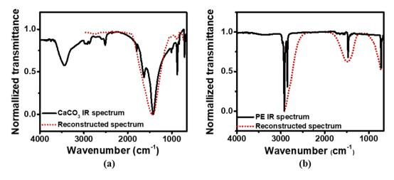
**Figure 5.** (a) FTIR spectrum of CaCO<sub>3</sub> (solid) and reconstructed spectrum (dotted); (b) FTIR spectrum of polyethylene (solid) and reconstructed spectrum (dotted).
