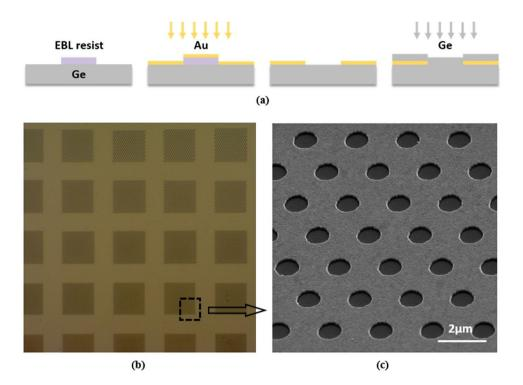
**Figure 2.** (a) Fabrication process of Au microhole arrays. Step I: applying EBL to write patterns in ZEP520 on Ge. Step II: depositing an 80 nm-thick Au film via electron beam evaporation. Step III: using acetone to pattern Au film. Step IV: sputter a 160 nm-thick Ge layer on the top of metal. (b) Overview micrograph of Au microhole arrays. (c) A close-up SEM image of the fabricated Au microhole array on Ge wafer.
