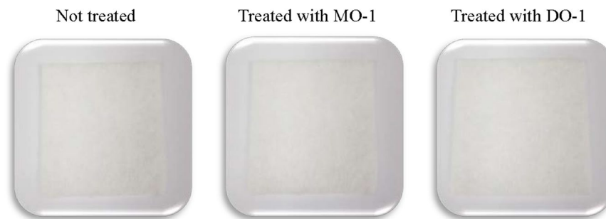
Figure 3. Staining effect of spray formulations on white cotton. Each test sample was then sprayed two times successively at 15 cm upwards.
