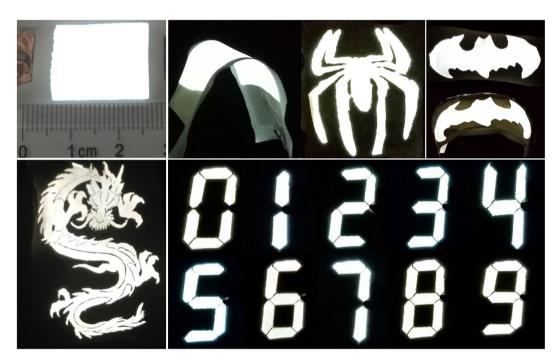
**Figure 3.** Photographs of the large-area flexible device. The flexible device under flat and mechanical bending state with different size and shape patterns.
