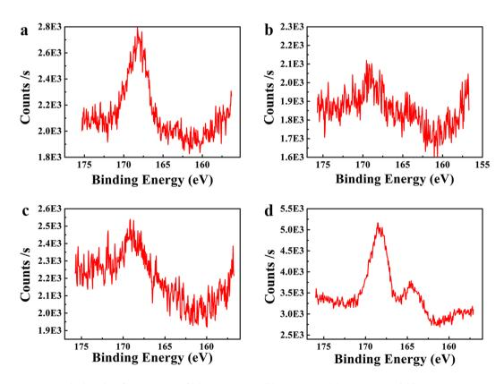
**Figure 6.** S(2p) peaks of XPS spectra of (**a**) PEDOT:PSS, (**b**) P-RGO-10, (**c**) P-GO-10, and (**d**) P-GQDs-10.
