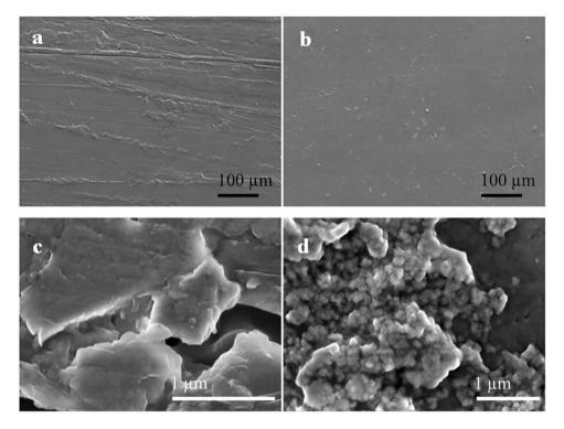
Figure 3. SEM images of PEDOT:PSS (a,c) and P-GQDs-10 (b,d).
