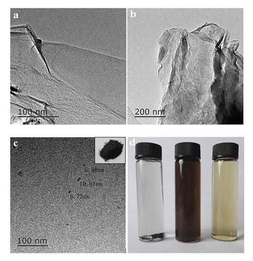
**Figure 2.** TEM images of (**a**) GO, (**b**) RGO, and (**c**) GQDs (inset image is GQDs powder). (**d**) their waterdispersing behavior (1 mg/mL) after an ultrasonic treatment for 30 days (left: RGO, middle: GO, right: GQDs).
