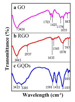
Figure 1. FTIR spectra of (a) GO, (b) RGO, and (c) GQDs.
