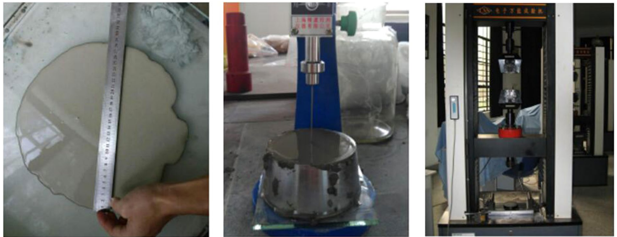
(a) Pumpable time test (b) ISO standard Vicat Apparatus (c) CSS44100 electronic universal testing machine
