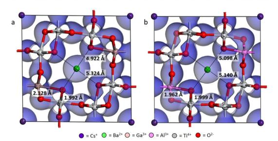
**Figure 6.** Ball and stick models of intermediate (**a**) Ga-hollandite and (**b**) Al-hollandite with the electron density projection overlaid in blue. Average bond distances are noted. Oxygen is red, Ti is grey, Ga is peach, Al is pink, Cs is purple, and Ba is green.
