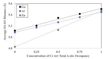
**Figure 5.** Average O1-O1 distance plotted against concentration of Cs for Ga- and Al -hollandite. Dotted lines are a linear fit to the data with a fixed intercept at the Ba-end member average O1-O1 distance.
