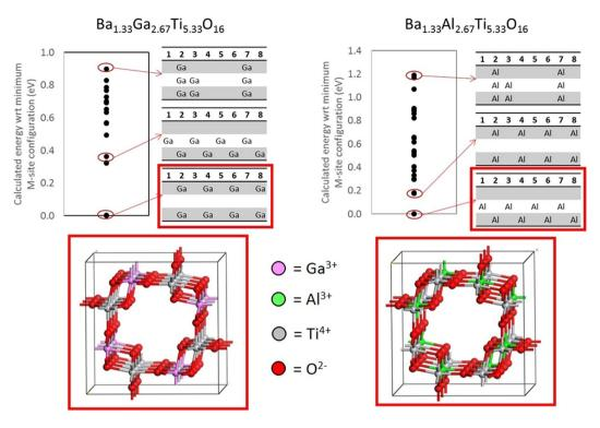
**Figure 3.** Range of energies for the Ba-end member compositions for Ga- and Al-hollandite with the configuration chart highlighted for the optimal configuration (lowest energy), an intermediate configuration, and the highest energy configuration. The ball and stick models show the lowest energy arrangement of the Ga (pink) and Al (green) B-site dopants. Note: Ti (grey), O (red), and A-site cations removed for clarity.
