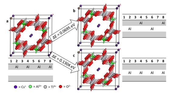
**Figure 4.** Impact of B-site ordering on the total energy of the Al-hollandite system demonstrated with balland-stick models, configuration charts, total energies, and change in energy with respect to the lowest energy configuration (**a**), where (**b**) shows the impact of a slight change in the B-site ordering and (**c**) shows the impact of the relative position of B-site and A-site cations. Cs (purple), Al (green), Ti (grey), O (red).
