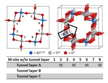
**Figure 1.** Schematic representing the B-site tunnel with the B-sites numbered within a tunnel layer, the tunnel layers labeled A, B, and C, and a configuration chart describing the B-site configuration. O (red), Ti (grey), M (blue).
